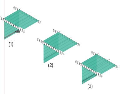
During fire the screen fabric has a tendency to shrink. Make sure that both the back edge and the leading edge will not come loose during fire, but remain connected to the leading edge profile or tube and truss or steel support wire.
