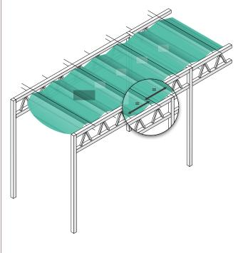
\* Note: make sure that the leading and the back edge side of the screen remain parallel in order to avoid wrinkles.
