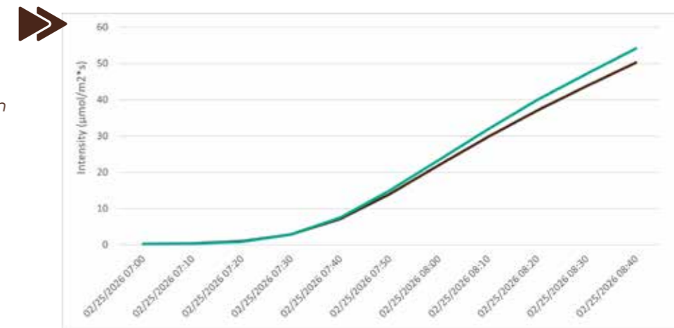
Graph 11: Change in light intensity beneath Diamond (green) and a traditional energy screen (brown) between sunrise and the opening of the screen, measured on February 25, 2026. Measured by Proefcentrum Hoogstraten.
