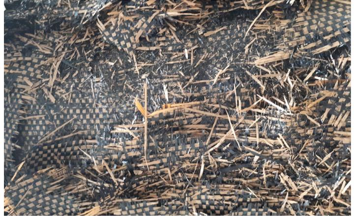
*Degraded Duracover after greenhouse test*
