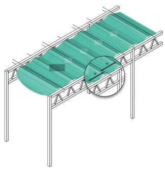
\* Note: make sure that the leading and the back edge side of the screen remain parallel in order to avoid wrinkles.
