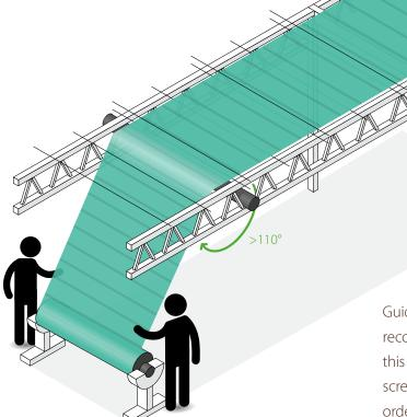
Make sure that the angle is greater than 110° and the screen is pulled over a smooth, plastic tube (minimum  $\emptyset$  125 mm) for minimum friction.
