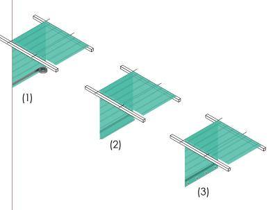
During fire the screen fabric has a tendency to shrink. Make sure that both the back edge and the leading edge will not come loose during fire, but remain connected to the leading edge profile or tube and truss or steel support wire.
